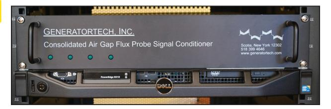
**Generatortech's G50 System** advances the technology of monitoring the health of generator field windings with a permanent connection to your generators. The G50 provides accurate real-time monitoring for continuous or periodic recording of flux probe data for evaluation of rotor winding shorted turn conditions.
